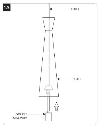
1 Feed the cord and socket assembly through the shade.
