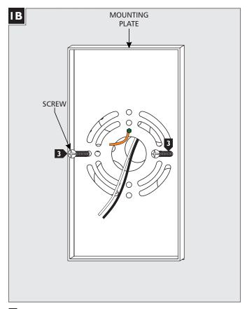
Attach the mounting plate to the electrical box using the two #8-32 screws provided.
