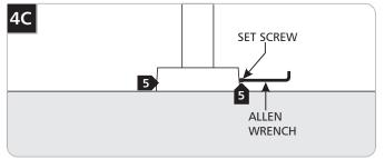
Carefully place the power line/cord inside the fixture, install the fixture onto the base plate, and secure it in place by tightening down the set screws.
