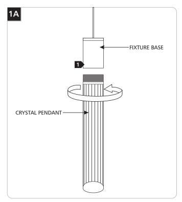
1 Screw the crystal pendant completely into the fixture base.
