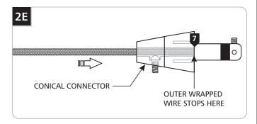
7 Feed and push the coaxial cable into the conical connector. The coaxial cable will come to a stop point after being inserted 3/4" into the conical connector.
