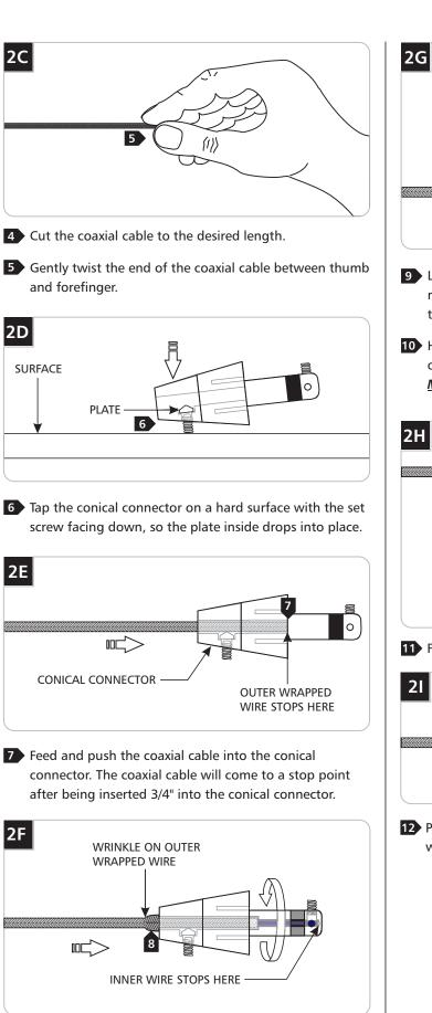
8 Keep pushing the coaxial cable into the connector while rotating the connector to ease feeding the inner wire into the tip of the connector. The outer wrapped wire will start wrinkling while being inserted another 1/2" into the connector.
