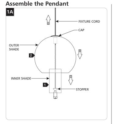
Feed the fixture cord through the inner shade then gently rest the inner shade on the stopper.
