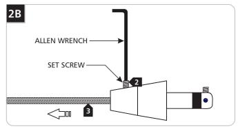
**2** Back out (do not remove) the set screw on the conical connector with the provided Allen wrench.
