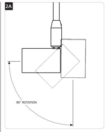
1 Rotate the socket up to 90°.
