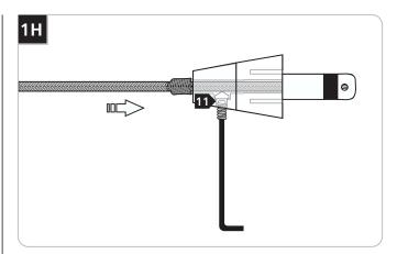
11 Firmly tighten the set screw on the conical connector.
