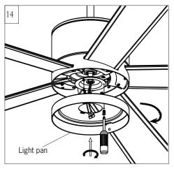
Attach light pan onto the plate on motor, Place light pan over the lead wires from fan, aligning the keyhole slots on the light plate with the preassembled screws on the plate. Twist clockwise till lock. Reinstall the screw remove in installation step 13. Tighten all screws securely.
