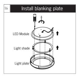
Remove LED module and Light shade from Light plate as shown in illustration. Keep screws.
