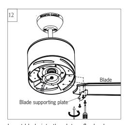
Insert blade into the slot on flywheel. Install blade with a blade supporting plate by the screws provided, aligning each of the holes as shown and tighten all screws securely. Repeat this process for remaining blades.
