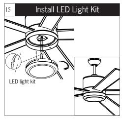
Connect white wire from fan to white wire from LED light kit and then connect blue (or black) wire from fan to black (or blue) wire from LED light kit.
