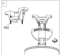
Lift Canopy, allowing the 2 studs to protrude through the canopy. Install knurled nuts provided and tighten the knurled nuts securely. The canopy should adjust for any irregularity in the ceiling or outlet box.
