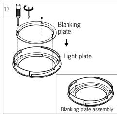
Install blanking plate onto light plate using the set screws of light shade which were just removed.
