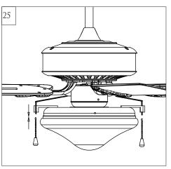
Thread pull chains through pull chain guides, and Install pull chains to preassembled pull chains on fan. Pull chains provided.
