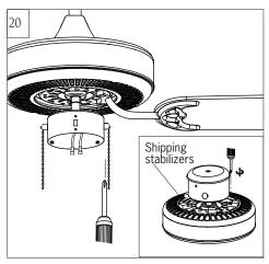
Remove shipping stabilizers from motor assembly.
