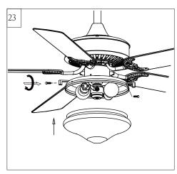
Partially loosen 3 set screws from light fixture.
