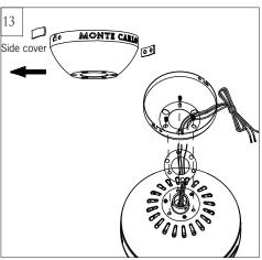
Remove side covers from canopy exposing 4 holes. 2 closed holes and 2 open "L" shape holes.
