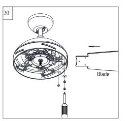
Insert blade into the slot on flywheel. Install blade with screws and fiber washers provided, aligning each of the holes as shown and tighten all screws securely. Repeat this process for remaining blades.
