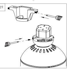
Install 2 of the screws to the side panel of mounting bracket corresponding to the open slotted holes on the canopy upper rim, screws provided. Remove the thread studs from the lower part of the mounting bracket.
