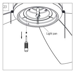
Loosen 2 and remove 1 preassembled screw from light pan. Save screw for later use.
