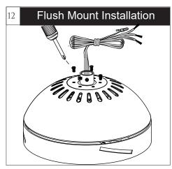
Remove every other screws from yoke located on top of fan assembly. Keep screws.
