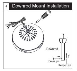
Partially loosen downrod set screws from yoke at top of motor assembly. Remove preassembled cross pin and keeper pin from downrod. Save parts.
