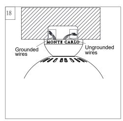
After making the wire connections, the wires should be spread apart with the grounded conductor and the equipment-grounding conductor on one side of the outlet box and ungrounded conductor on the other side of the outlet box. The splices after being made should be turned upward and pushed carefully up into the outlet box.
