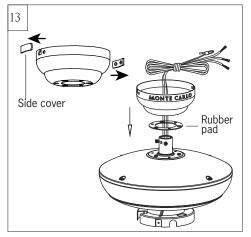
Remove side covers from canopy exposing 4 holes. 2 closed holes and 2 open "L" shape holes.
