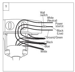
Make wiring connections using wire connectors provided as indicated above. White from fan to White (Neutral) from house. Black and Blue from fan to Black (Live) from house. Connect all green grounded wires to Grounded wire from House. Make sure that no filaments are outside of the wire connectors.
