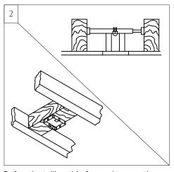
Before installing this fan make sure the outlet box is properly installed to the house structure. To reduce the risk of fire, electric shock, or personal injury, mount to outlet box or supporting system acceptable for fan support.
