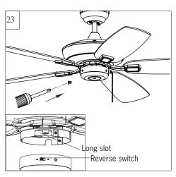
Align the long slot on top plate with the reverse switch on switch housing, and then install the switch housing onto the top plate with the 3 set screws removed in step 21 and tighten all screws securely.
