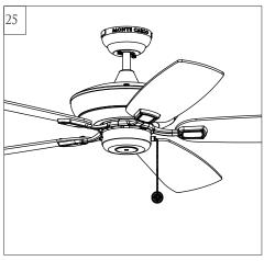
Install fan pull chain to preassembled pull chain on fan. Pull chain provided.
