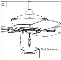
Connect the plug from fan with the plug from switch housing. Be sure plugs connection clasped together completely.
