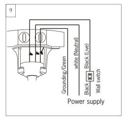
Make wiring connections using wire connectors provided as indicated above. Connect Black wire from fan to Black (Live) wire from house. Connect White wire from Fan to White (Neutral) wire from house. Connect all green grounded wires to Grounded wire from House. Make sure that no filaments are outside of the wire connectors.
