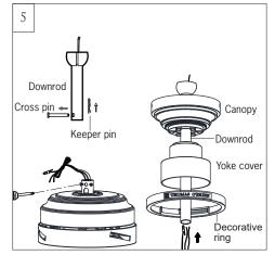
Partially loosen downrod set screws from voke at top of motor assembly. Remove preassembled cross pin and keeper pin from downrod.
