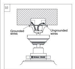
After making the wire connections, the wires should be spread apart with the grounded conductor and the equipment-grounding conductor on one side of the outlet box and ungrounded conductor on the other side of the outlet box. The splices after being made should be turned upward and pushed carefully up into the outlet box.
