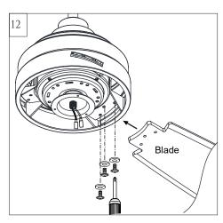
Insert blade into the slot on flywheel. Install blade with screws and washers provided, aligning each of the holes as shown and tighten all screws securely. Repeat this process for remaining blades.
