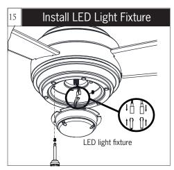
Connect white wire from fan to white wire from LED light fixture and then connect blue (or black) wire from fan to black (or blue) wire from LED light fixture. Be sure plugs connection clasped together firmly. Attach LED light fixture onto the light pan, aligning the keyhole slots on the LED light fixture with the preassembled screws on the light pan. Twist clockwise till lock. Reinstall the screw which was just removed. Tighten all screws securely.
