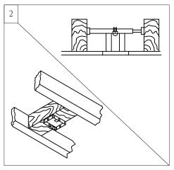
Before installing this fan make sure the outlet box is properly installed to the house structure. To reduce the risk of fire, electric shock, or personal injury, mount to outlet box or supporting system acceptable for fan support.
