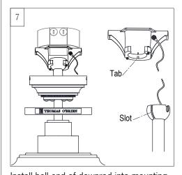
Install ball end of downrod into mounting bracket opening. Align (engage) slot on ball with tab on mounting bracket. **Warning:** Failure to align slot on ball with tab may result in serious injury. **Important:** If using the angle mount, make sure open end of mounting bracket
