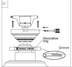
Raise canopy to mounting bracket, aligning loosened screws in mounting bracket with slotted holes in canopy. Twist canopy clockwise to lock. Reinstall screws that were previously removed in step 3 and then tighten all screw securely.
