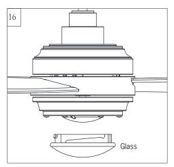
Attach glass by locating dimples in light pan with grooves on the glass and twist clockwise until tight.
