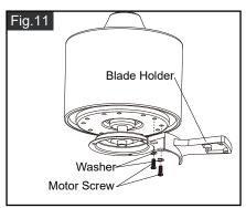
Remove the motor screws and washers from the motor assembly. Secure blade holders to the motor with washers and motor screws.
