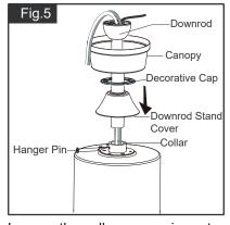
Loosen the collar screws in part way. Insert the Downrod into the Collar. Slide Hanger Pin through holes of Collar and Downrod.
