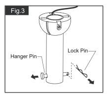
Remove the Lock Pin and take off the Hanger Pin.
