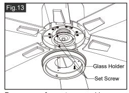
Remove one fan motor assembly screw (for later use), Push the glass holder upwards until the fan motor assembly screws insert into the key hole slot of glass holder then rotate the glass holder till it fixed on the motor bottom. Finally, secure the glass holder to motor bottom with previous screw which we removed and tighten the other two fan motor assembly screws.
