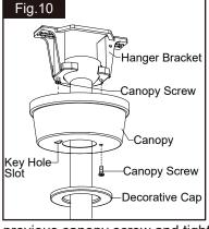
Remove one canopy screw (for later use), then push the canopy upwards by inserting canopy screw head left in hanger bracket into key hole slot, rotate the canopy till the hole in canopy aligns the hole in hanger bracket, finally, secure the canopy to hanger bracket with
