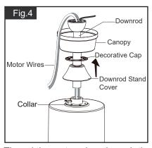
Thread the motor wires through the downrod stand cover, decorative cap, canopy and downrod.
