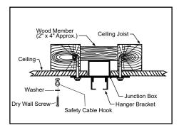
Tighten the hanger bracket to the outlet box with two mounting screws.(Make sure the outlet box is securely installed so that it will be able to support at least the fan weight.) Attach the safety cable hook to the ceiling with the dry wall screw and washer, and make sure the safety cable hook is covered by the fan canopy.
