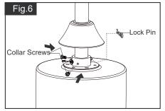
Insert and tighten the two Collar Screws. Slide Lock Pin into Hanger Pin until it is locked into position.
