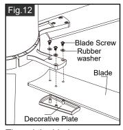
Thread the blade screws through the rubber washer, blade holder and blade into the decorative plate. Tighten all blade screws securely. Repeat to other blades.
