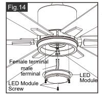
Connect the female terminals from motor to male terminals from LED module.
