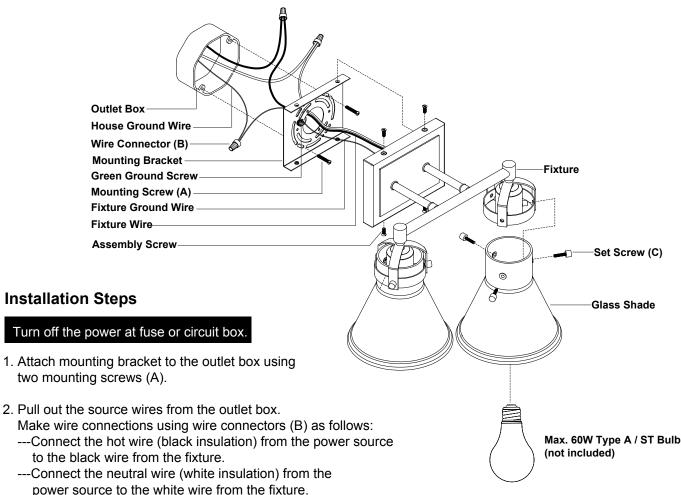
Carefully put the wires back into the outlet box.
