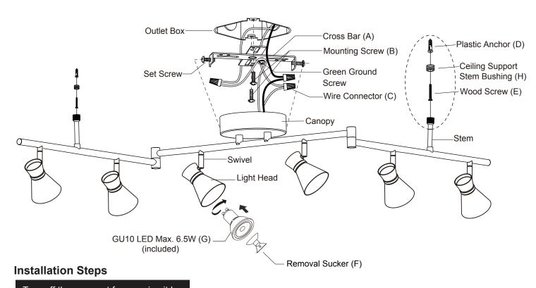
Turn off the power at fuse or circuit box
