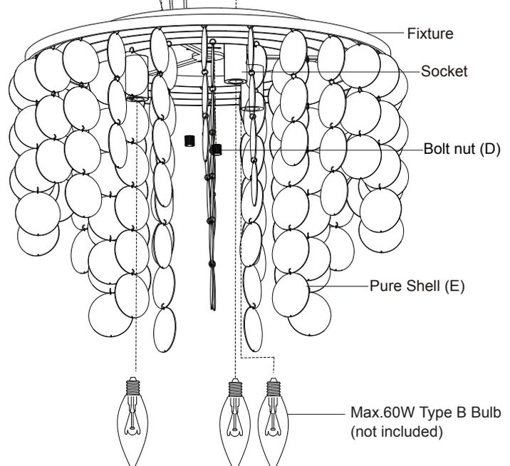
6. Install bulbs (not included). See relamping label at socket area or packaging for maximum allowed wattage.
