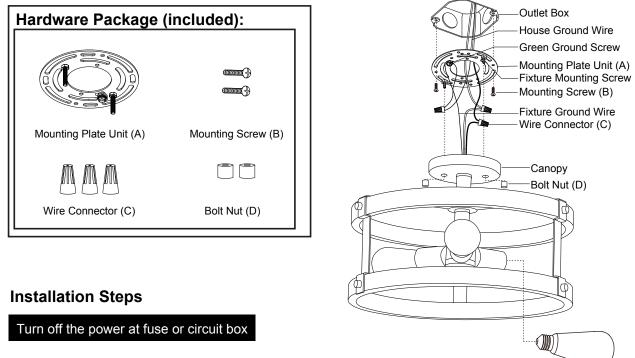
1. Attach the mounting plate unit (A) to the outlet box by using two mounting screws (B).
