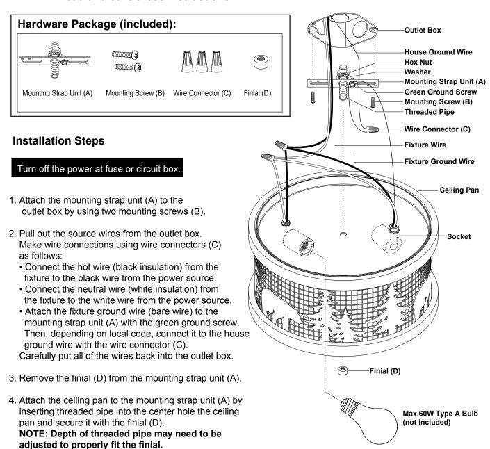
6. Install 2 x 60W max. medium base bulbs (not included). Check relamping label at socket area or packaging for maximum wattage allowed.
