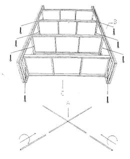
2.Unfold the two side shelves (B) carefully, and let the whole wooden shelves (C)stand on the floor.
