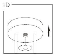
Lining up threads on crossbar with hole in backplate, attach fixture to junction box using cap nut. Be sure to carefully tuck wires into backplate while attaching.
