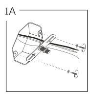
Carefully pull house wires out of junction box. With threads facing outward, screw crossbar into junction box using outlet box screws.
