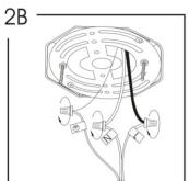
Strip 3/4" of insulation from wire ends. Connect house ground wire to fixture ground wire marked with symbol. Twist wires together using wire nut. Connect black house wire to the fixture wire marked "L". Twist wires together using wire nut. Connect white house wire to the fixture wire marked "N". Twist wires together using wire nut.
