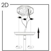
Lining up threads on mounting plate with holes in fixture canopy, attach fixture to junction box using cap nuts. Be sure to carefully tuck wires into canopy while attaching.
