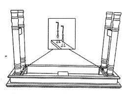
Put the table top upside down on soft & clean surface. Attach metal leg to the bottom of the table top with bolts" F ", flat washers and Allen wrench "H" as shown above. Please don't fully tighten bolts.
