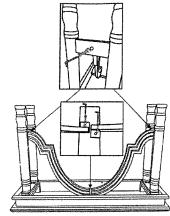
Attach wooden supporter to the unit with bolts "F", flat washers and Allen wrench "H".Please don't fully tighten bolts.
