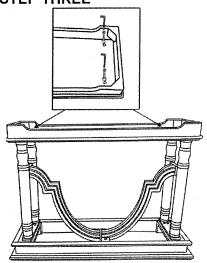
Attach wooden base to the end of leg with bolts "G", flat washers and Allen wrench "I".
