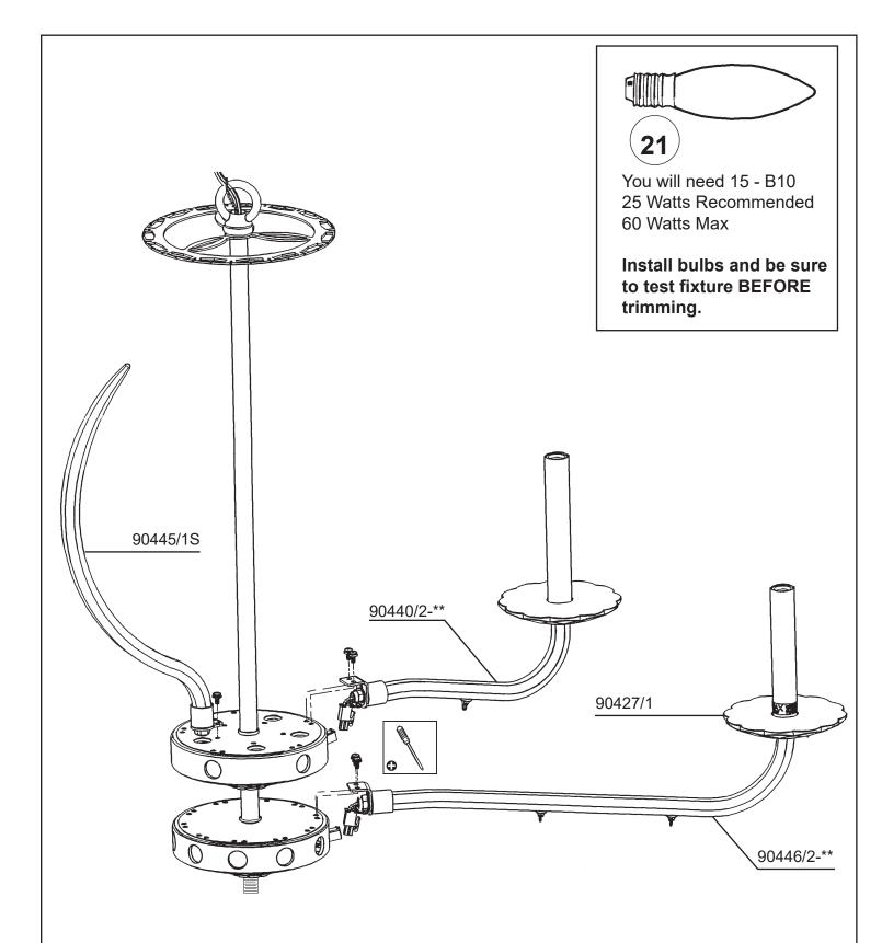
19 Connect arm wires using plug-in connectors on top and bottom tiers. See detailed illustration.
