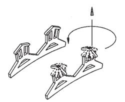
**A** Turn both tabs 90° counterclockwise on either side of pocket where the octagon should be.
