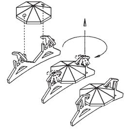
**B** Slide crystal octagon into pocket. Turn both tabs clockwise back to original position to hold the octagon in place.
