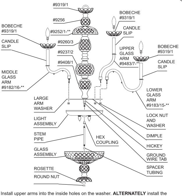
**8** Install upper arms into the inside holes on the washer. **ALTERNATELY** install the middle and lower arms into the outside holes on the washer. NOTE: THE **FIRST** LOWER ARM INSTALLED SHOULD LINE UP WITH A UPPER ARM. Line up holes in arms with dimple in washer. Use lock washer and nut to secure arms in place. Unscrew nut on nipple, place ground wire tab over nipple, secure with nut.
