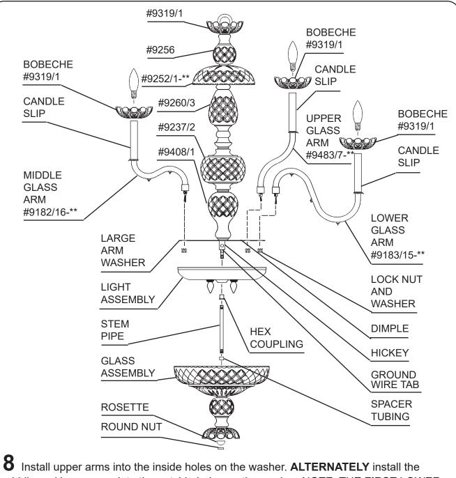
**8** Install upper arms into the inside holes on the washer. **ALTERNATELY** install the middle and lower arms into the outside holes on the washer. NOTE: THE **FIRST** LOWER ARM INSTALLED SHOULD LINE UP WITH A UPPER ARM. Line up holes in arms with dimple in washer. Use lock washer and nut to secure arms in place. Unscrew nut on nipple, place ground wire tab over nipple, secure with nut.
