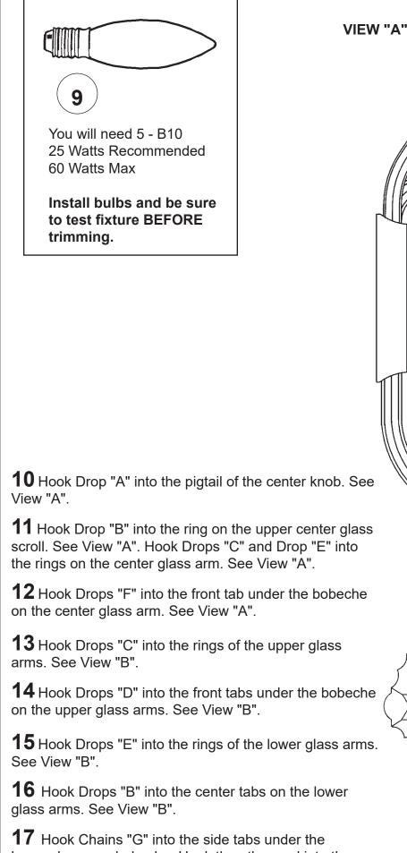
If Hook Chains "G" into the side tabs under the lower glass arm bobeche. Hook the other end into the side tabs under the center glass arm bobeche. Chains "G" are swagged between the center glass arm and the outside glass arms. See View "B".
