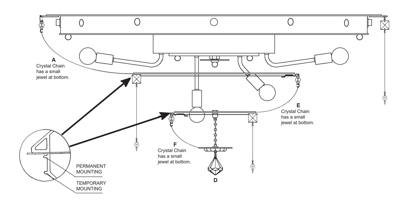
**8** Hang upper mirror Chains "A" FIRST. Hook all Chains "A" into holes in the outer ring so that the metal accessories face outwards and square jewel is on the upper end. Hook the loose end of Crystal Chains "A" with small jewels into holes of solid mounted metal ring.
