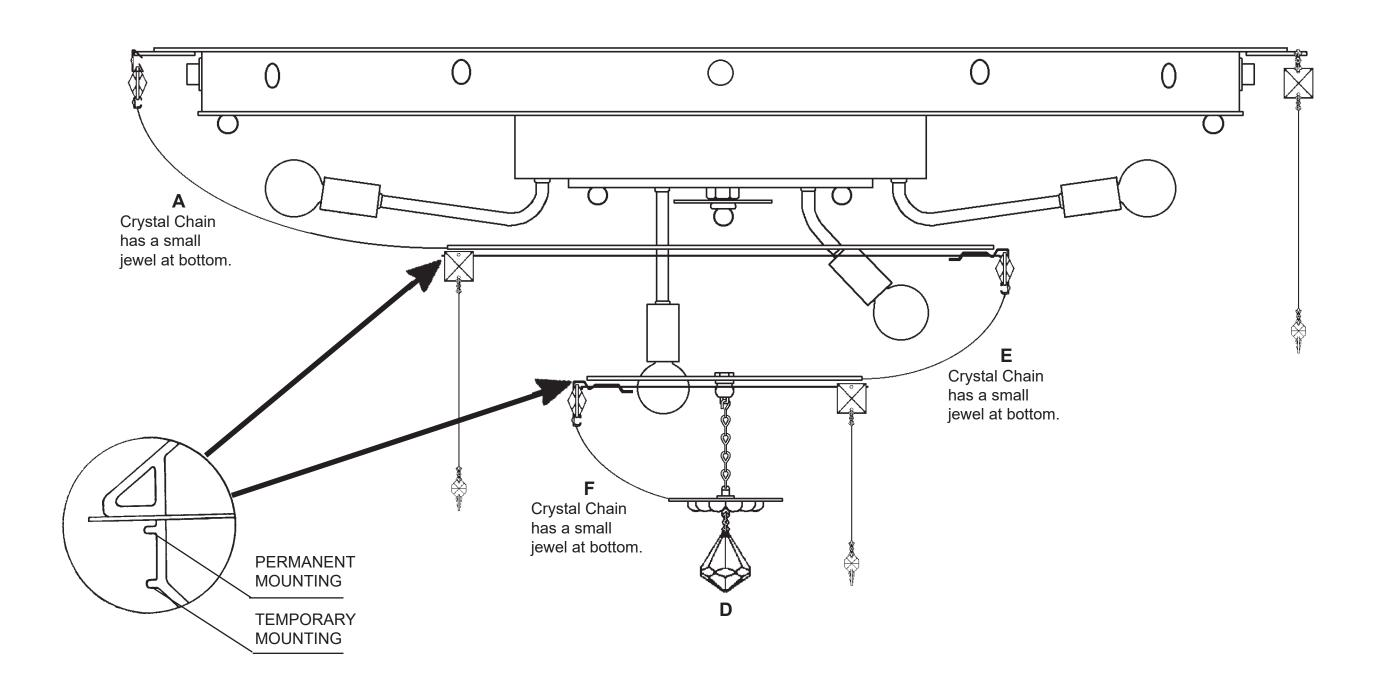
**9** Hang upper mirror Chains "A" FIRST. Hook all Chains "A" into holes in the outer ring so that the metal accessories face outwards and square jewel is on the upper end. Hook the loose end of Crystal Chains "A" with small jewels into holes of solid mounted metal ring.
