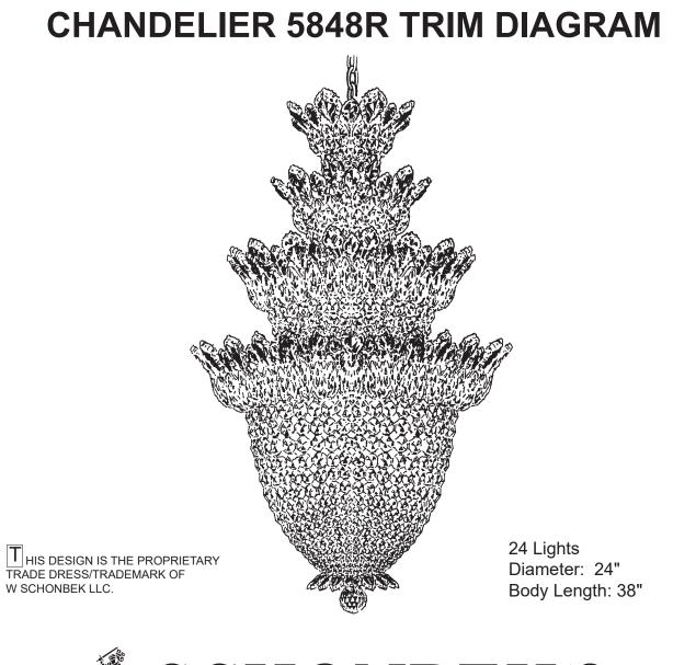
CAUTION... RISK OF ELECTRICAL SHOCK. Make sure the electrical supply to the chandelier is turned off at the main fuse or circuit breaker before doing any installation. All electrical components must be installed by a licensed electrician in accordance with the National Electric Code and the appropriate local electrical codes. HANGING WEIGHT: 45 pounds. BULBS: (24) Candle shaped candelabra base B10 bulbs, recommend 25 watts
