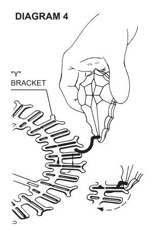
Position the crystal above the "Y" bracket so that the end of the hook enters the long slot, gently push toward the center of the fixture and raise the crystal making sure that the end of the hook comes up through the short slot, in line with the long slot.
