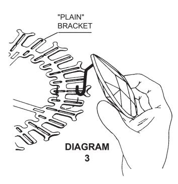
Position the crystal above the "plain" bracket so that the end of the hook enters the slot, gently push toward the center of the fixture and raise the crystal making sure that the end of the hook comes up through the inner slot, in line with the outer slot.
