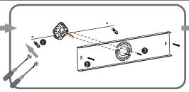
For drywall installations, insert wall anchors into the holes. Otherwise, secure crossbar assembly using self-tapping screws. Then, fully tighten the outlet box screws.
