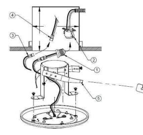
Install screw into correct mounting hole for appropriate recessed housing size.
