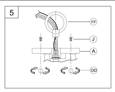
5. Pass the wires through the chain loop (FF). Then thread the chain loop (FF) onto the nipple at the top of the fixture (A). Tighten chain loop (FF) securely to the fixture (A).
