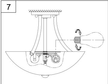
7. Thread the lamp (not included) into the fixture socket. Use 100-watt MAX incandescent medium base lamp, SBCFL or SBLED.
