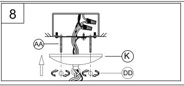
8. Pass the screws (AA) through the two holes in the canopy (K). Secure the fixture to the screws (AA) using the two ball nuts (DD). Tighten securely.
