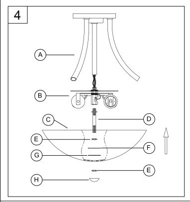
4. Pass the wires from the socket cluster (B) through the fixture (A). Tighten socket cluster (B) securely to the fixture (A).
