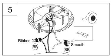
5. Strip 3/8" of insulation from the electrical wire ends. Using wire nuts (BB), connect RIBBED fixture wire to the WHITE supply wire from the outlet box; connect the SMOOTH fixture wire to the BLACK supply wire.
