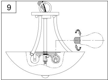
9. Thread the lamp (not included) into the fixture socket. Use 100-watt MAX incandescent medium base lamp, SBCFL or SBLED.
