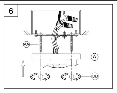
6. Pass the screws through the two holes in the canopy. Secure the fixture (A) to the screws (AA) using the two ball nuts (DD). Tighten securely.
