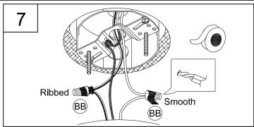
7. Strip 3/8i± of insulation from the electrical wire ends. Using wire nuts (BB), connect RIBBED fixture wire to the WHITE supply wire from the outlet box; connect the SMOOTH fixture wire to the BLACK supply wire.
