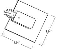
NT-352B: Black Live End Feed with Canopy NT-352S: Silver Live End Feed with Canopy NT-352W: White Live End Feed with Canopy
