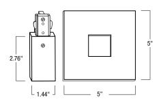
NT-311B: Black Live End Feed with Canopy NT-311S: Silver Live End Feed with Canopy NT-311W: White Live End Feed with Canopy
