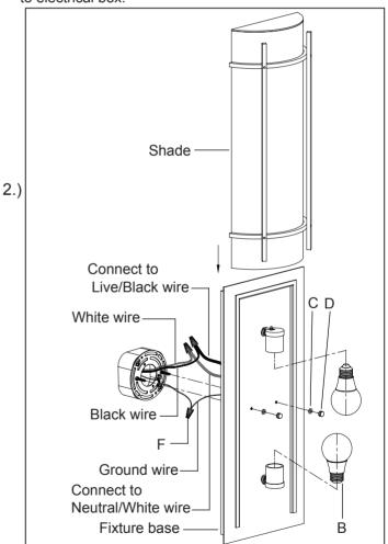
Step2:Wire fixture to wires in outlet box.Copper wire is for Ground.Attach Fixture base to mounting bracket and tighten with Nuts (D).Screw light bulbs(included) into the socket. Fit the shade onto the Fixture base.
