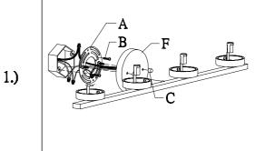
Step.1:Remove mounting bracket (A) from fixture and install to electrical box. Then wire fixture to wires in outlet box. Copper wire is for Ground. Attach backplate(F) to mounting bracket(A) and screws, then tighten by finial(C), so fixture meets wall.
