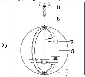
Step2. Adjust the flat metal by level at first, put the glass(G) on the cup, then secured by socket ring(F)
