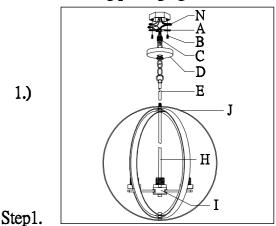
Remove crossbar from fixture and install to electrical box.
