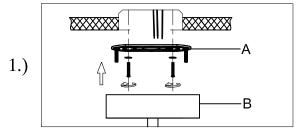
Step.1: Remove mounting bracket (A) from canopy (B) and install to electrical box.
