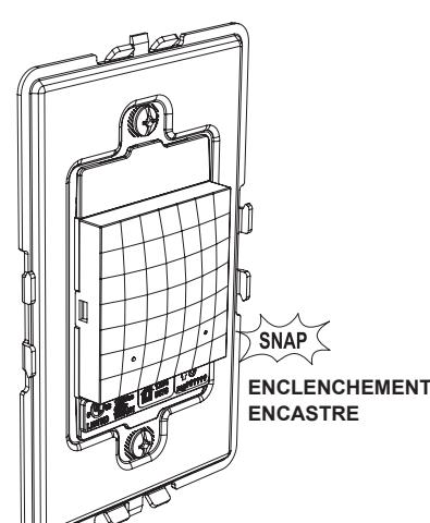
**TIP - Since the frame completes the enclosure, it's safe to power up the gateway and test. Allow one minute for the electronics to charge after installation.**
