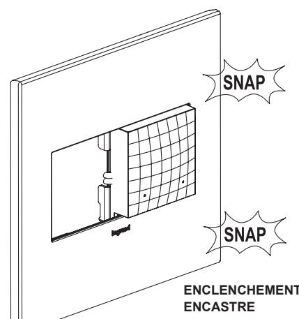
**NOTE:** To remove wall plate, insert a small, flat screwdriver in notches on wall plate and twist gently to pry from frame.
