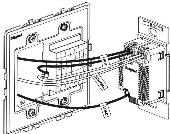
Connect the Hot Wire to the Black wire of the Gateway (follow instructions for mating device Hot connection).
