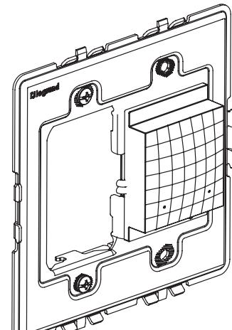
**NOTE:** If you need to remove mating device after snapping into frame, first remove frame from wall box to access the locking tabs on the back of the device. Insert a flat screwdriver to depress tabs as you apply pressure to push device out.
