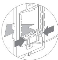
Determine if spacers are required for mating adorne™ device. To remove spacers, from the back of the frame, pinch the tabs on the spacer to release.
