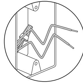
Connect frame ground wire to bare ground wire in box. Fold ground wires into back of box. Mount frame to wall box with screws provided with the Gateway portion hanging over the wall. Tighten screws just enough to hold frame in place. Do NOT overtighten.
