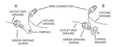
Make wire connections. Reference chart below for correct 3) connections and wire accordingly.
