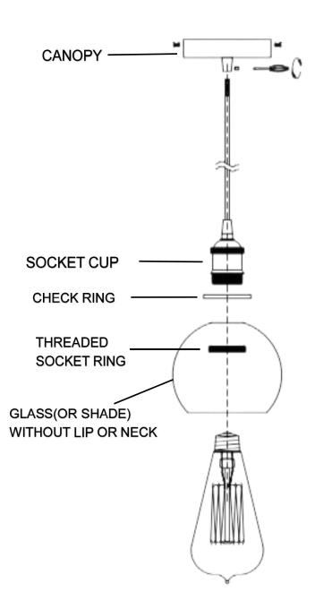
CHOOSE THE WIRE NEEDED FOR THE CEILING HEIGHT, THEN FEED THE WIRES INTO THE CANOPY, THEN USE A SCREWDRIVER TO SCREW THE PLASTICSCREWS IN TO SECURE THE WIRES, AND THE PLASTIC STRAIN RELIEF IN THE CANOPY IS ALSO FIXED THROUGH THE WIRES.
