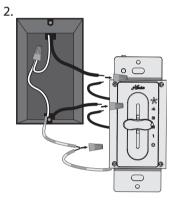
Installing the Wall Control
