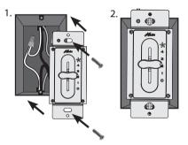
Mount the faceplate (not included) to the wall control using the two #6-32 screws (not included).
