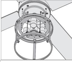
Lift cage assembly into place while passing pull chains through cage assembly as shown. Align the keyhole slots in the top of the cage assembly with the partially installed cage assembly screws. Wrap the keyhole slots around the screws and twist counterclockwise.
