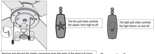
Remove and discard the plastic connectors from the ends of the short pull chain. Attach the pull chain pendants to the light and fan pull chains.
