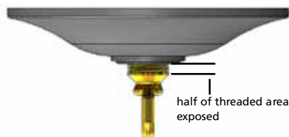
Drawing 2 Canopy Adjustment
