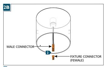
Remove the female fixture connector from the male connector.
