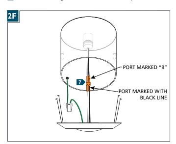
Reconnect the top and bottom socket adaptor terminals. NOTE: To ensure proper connection, the connectors have been marked with the letter B and a black line.
