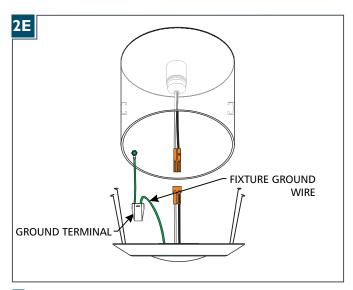
6 Insert the fixture ground wire to an available port.
