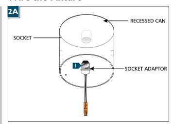
I Screw the socket adaptor into the socket.
