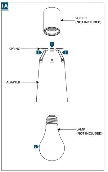
Install the adapter over the socket (**not included**) by snapping the springs onto the socket.
