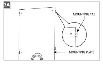
If necessary, carefully bend the mounting tabs 90 degrees as shown.
