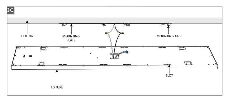
6 Neatly place all wires into the junction box or wiring compartment, align the mounting tabs to the slots on the fixture, push the fixture so that the tabs enter the slots and slide the fixture left or right depending on mounting tabs orientation to lock in place. Make sure THE fixture is fully secured before releasing.
