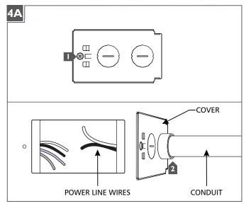
Remove the screw on wiring compartment cover located on the back of the fixture and remove cover completely.
