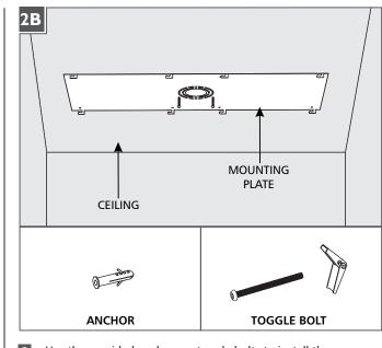
2 Use the provided anchors or toggle bolts to install the mounting plate to the ceiling according to local building code.
