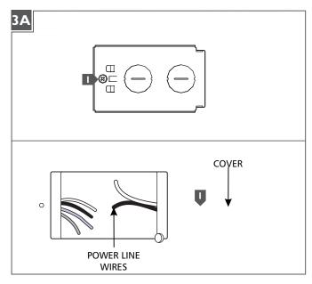
Remove the screw on wiring compartment cover located on the back of the fixture and remove cover completely.
