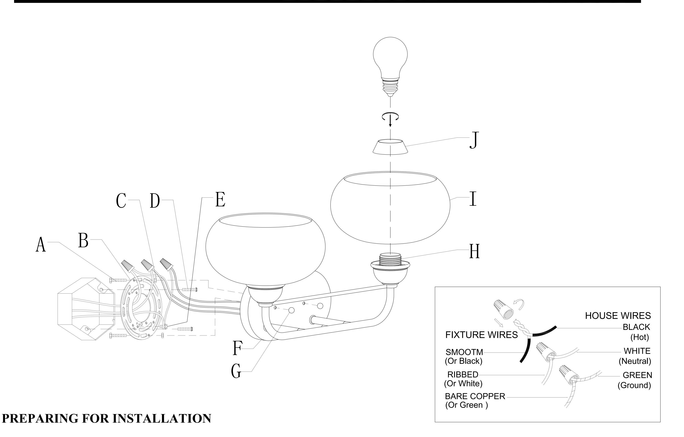
Remove all contents from the carton. See the important illustrations above. Shut off the power at the circuit breaker and completely remove the old fixture from the ceiling, including the old mounting strap.
