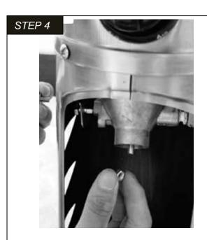
4-1. Fix the regulator to the tank housing with the M5x10mm bolt and M5 nut.
